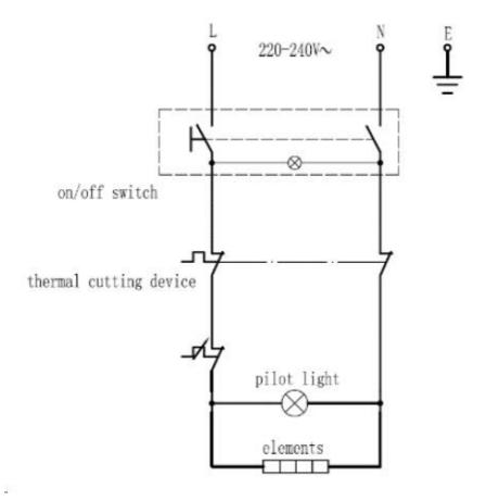
The above circuit diagram has been provided to assist qualified technicians, LINCAT agents or Recommended Qualified Technicians, should carry out repairs if needed. Do not remove any components or service panels on this product.
